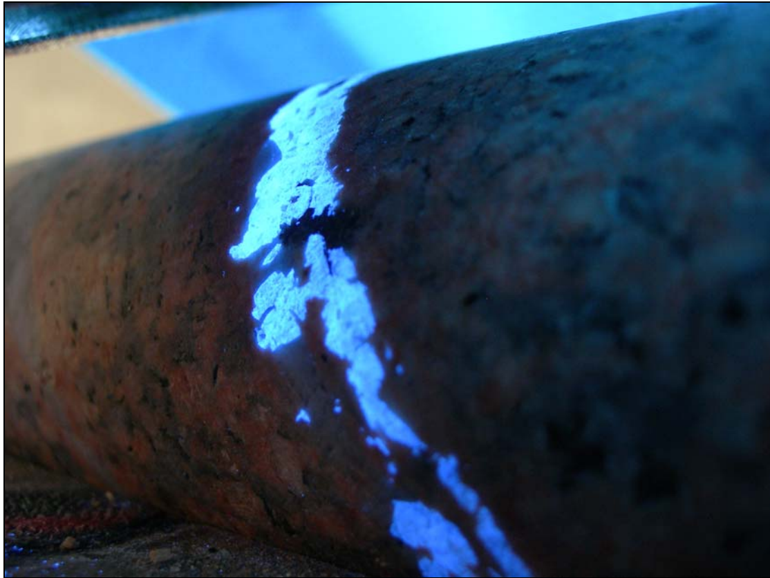
Figure 3: Tungsten mineral Scheelite in BAR-20 drill core. Scheelite is fluorescent and can be identified easily under ultraviolet light.
